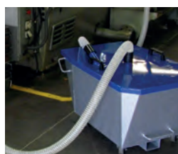
Sludge container Separated collection of sludges or shavings to wring
